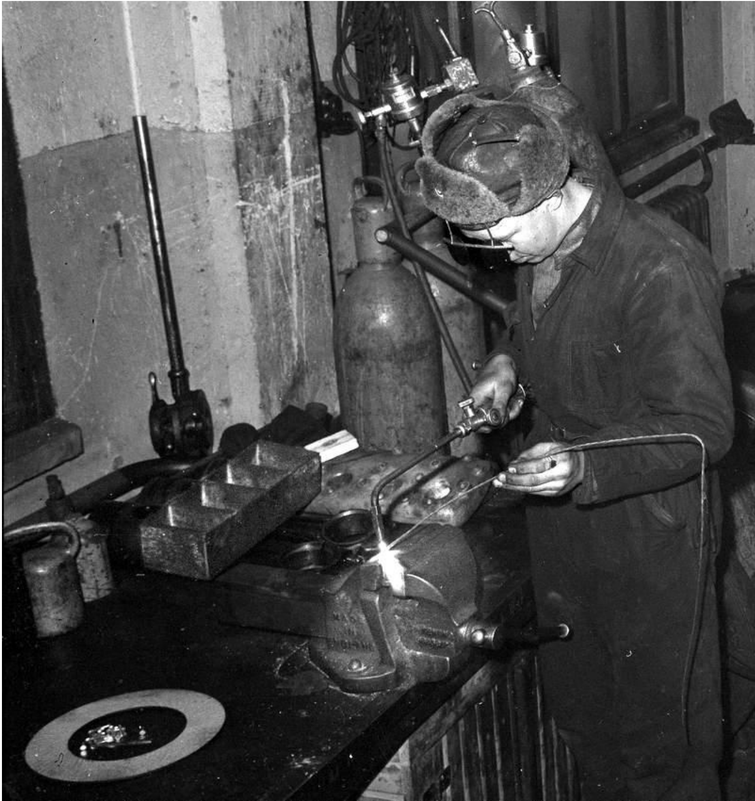
There is a (frozen?) broken engine head to be welded.
