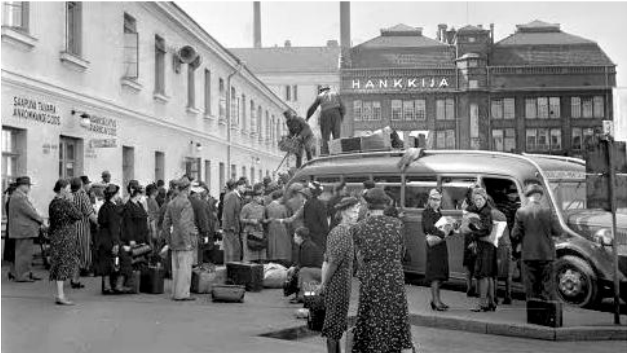
Helsinki Bus station. Bus: wood gasifier pipes ride on top, routed from rear to the engine.
